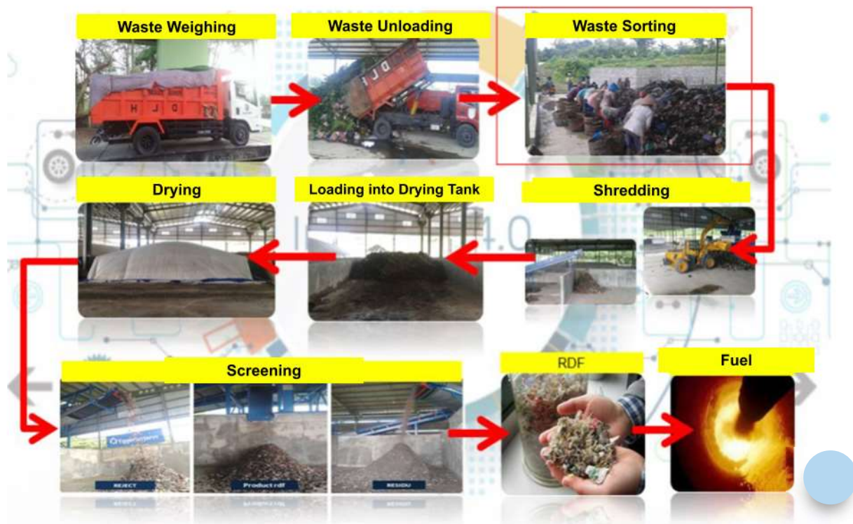
Figure 3.3 Waste Segregation as Part of the RDF Process in Kabupaten Cilacap Source: Environmental Agency of Kabupaten Cilacap
